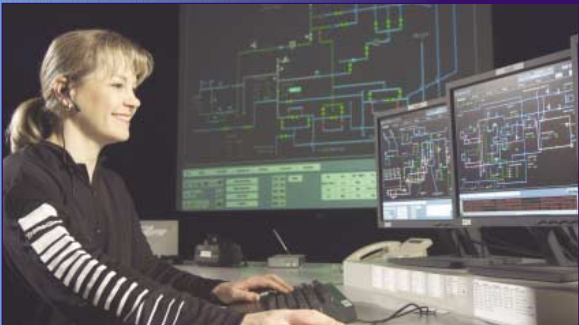
Donna Herchuk, Dispatcher for Gas Control, is one operator of the new Telvent SCADA (Supervisory Control and Data Acquisition) system that fully integrates gas control and information management systems within the Corporation.
